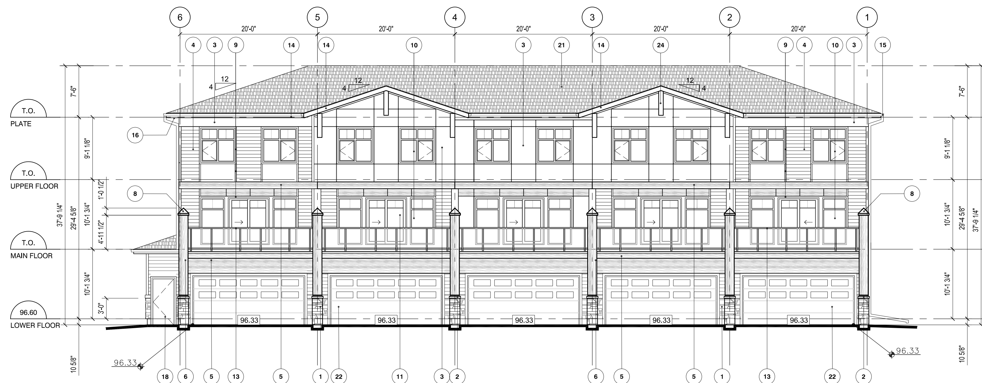
3 BACK BLOCK ELEVATION DP16 1/8"=1'-0"
