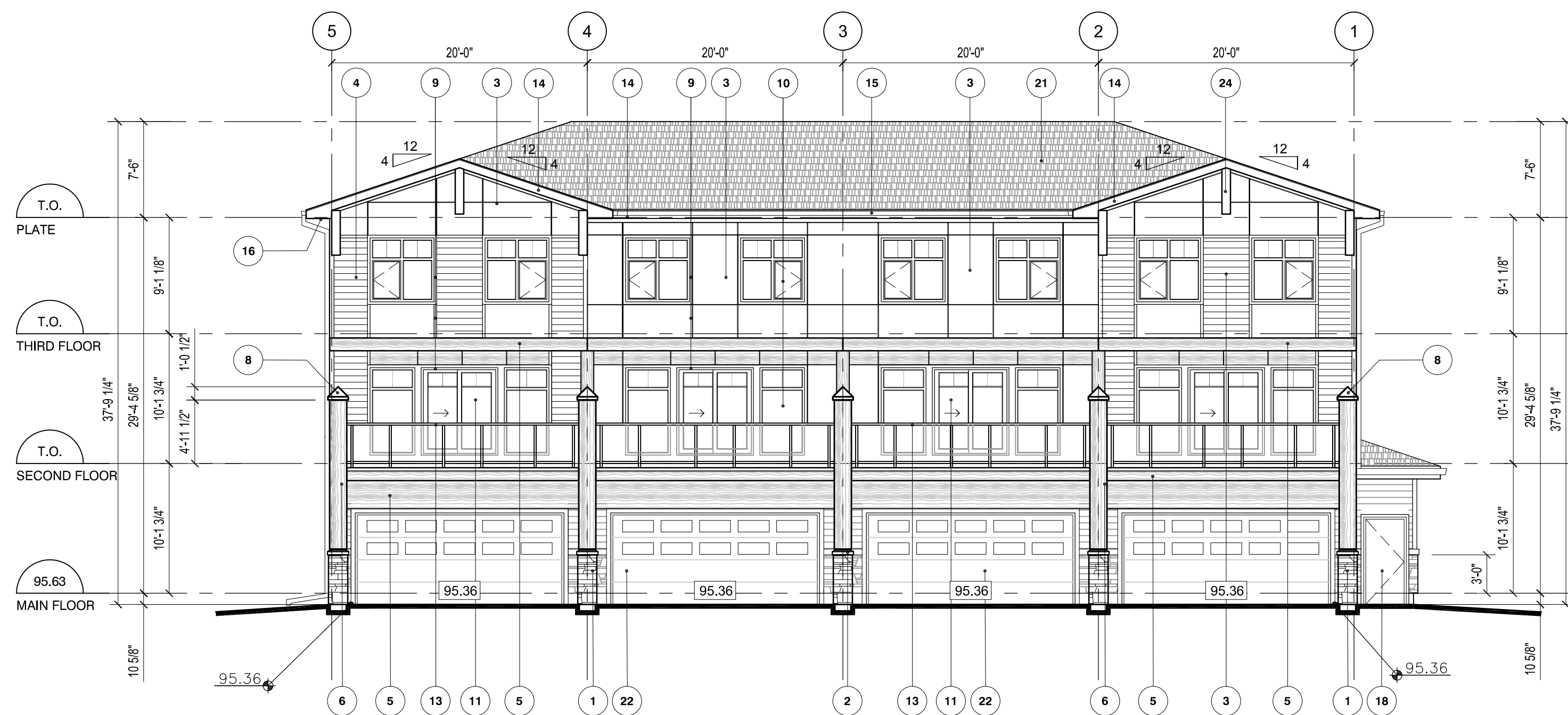
3 BACK BLOCK ELEVATION DP11 1/8"=1'-0"
